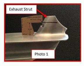
First, it is necessary to identify the lowest point of the allowable hole, which is 1.500" below the flat area of the cavitation plate. It is important to make sure you are measuring outside the radius at the bottom of the exhaust strut. Using your ruler, mark the leading edge of the strut and draw a line parallel to the cavitation plate. This line is the maximum limit of the hole. See Photo 1.
